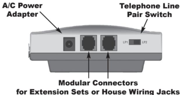
1. Connect the supplied A/C power adapter cord into the Dock-N-Talk™ round adapter plug shown above. Then connect the large transformer end into a normal 120-volt power outlet.
