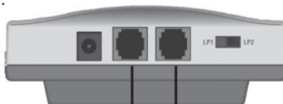
**Plug telephone line cord into one or both of Dock-N-Talk's modular telephone jacks**
